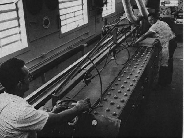
"STONE SAW" in Metal Stock and Cutting area can aluminum stock two inches thick, while Pedro S. Ortega
